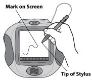
**IMPORTANT!** The mark made on your screen from the stylus and the location of the tip of the stylus may not align. When this happens, you need to calibrate the stylus.
