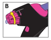
If ink foams at the tip, turn dial one click back towards the **starting position**. Clean any foam with a disposable cloth (not included) and test spray again. Repeat until spray no longer foams.
