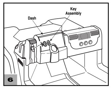
• Insert and "**snap**" the key assembly into the opening in the dash, as shown.
