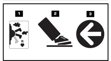
**IMPORTANT!** To avoid damaging the motors and gears, stop the vehicle before shifting from forward to reverse  $\clubsuit$ .
