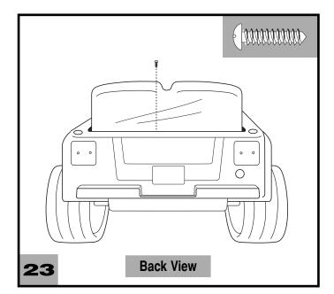
Insert a #10 x <sup>3</sup>/<sub>4</sub>" screw into the rear edge of the seat. Tighten the screw.
