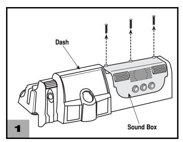
• Loosen and remove the three screws in the top of the sound box. Remove the sound box from the dash.
