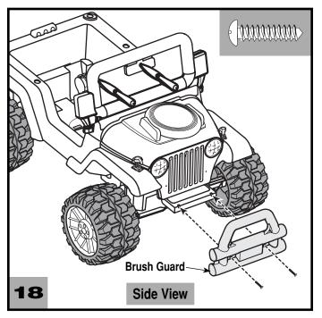
• Fit and hold the brush guard against the front end of the vehicle. *Hint:* Using the end of a Phillips screwdriver, poke a hole in the thin, plastic covering over the lower holes in the brush guard.
