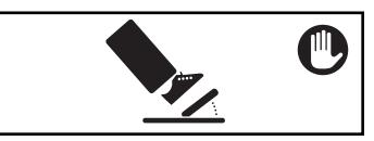
• Your vehicle has a patented, electronic braking system that automatically stops the vehicle when your child's foot lifts from the pedal. Make sure your child is comfortable with steering the vehicle and automatically knows how to stop.
