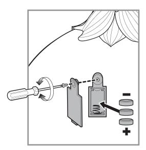
BATTERY REPLACEMENT: Requires 3-AG13 alkaline button cell batteries. Use a Phillips head screwdriver (not included) to open battery door. Insert 3- AG13 button cell batteries. Replace door and tighten screw. For longer battery life use only alkaline batteries. Replace batteries when the light dims.
